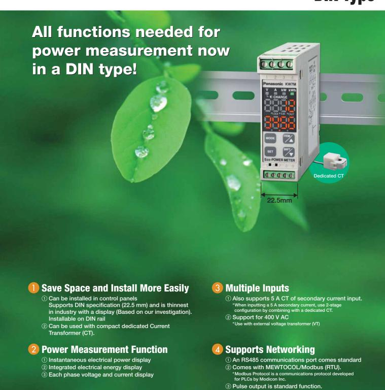
KW7M Eco-POWER METER DIN Type ARCT1B281E '07.6
